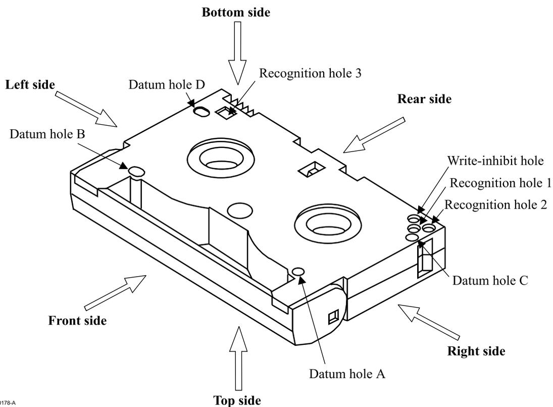
Figure 2 - Tape cartridge assembly, bottom view, lid closed
