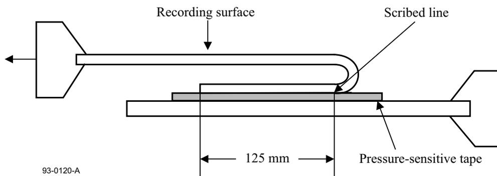
**Figure 27 - Measurement of the coating adhesion**
