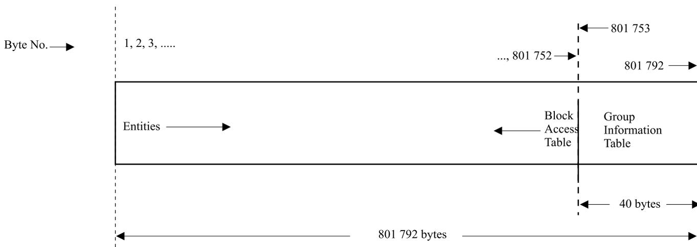
Figure 29 - Structure of a Basic Group
