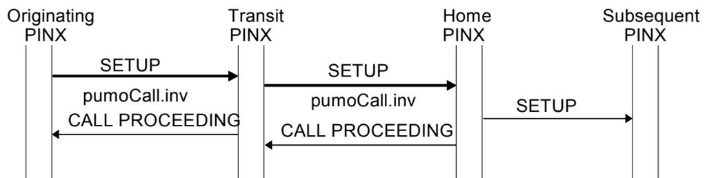
Figure C.7 - Successful invocation of ANF-PUMO with en-bloc operation
