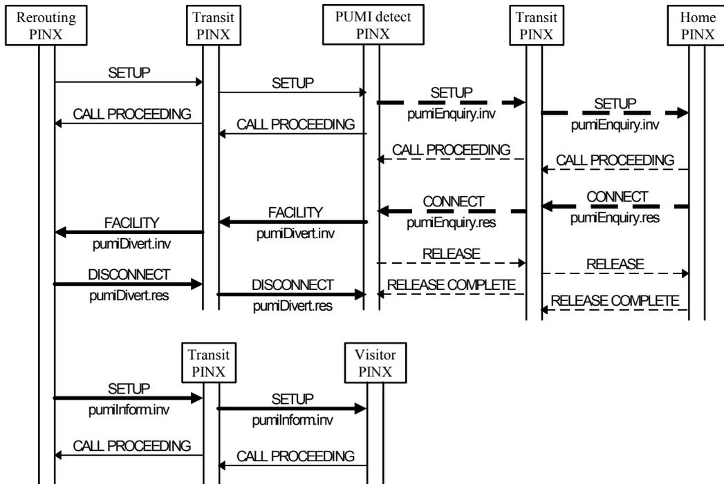
Figure C.1 - Example of normal operation of ANF-PUMI
