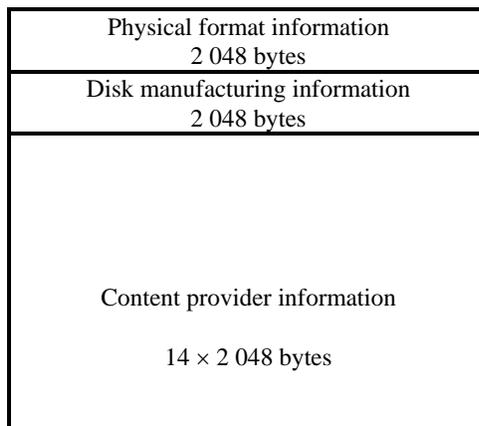
**Figure 28 - Structure of a Control Data Block**
