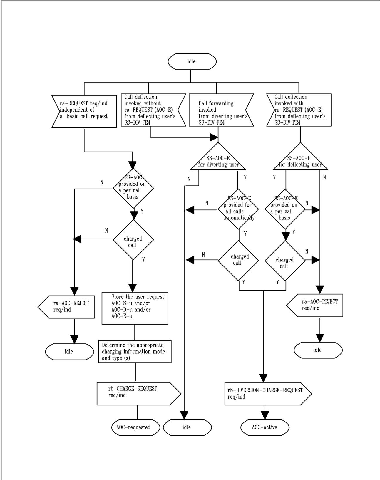
Figure 22 (part 2) - SS-AOC, SDL for functional entity FE2
