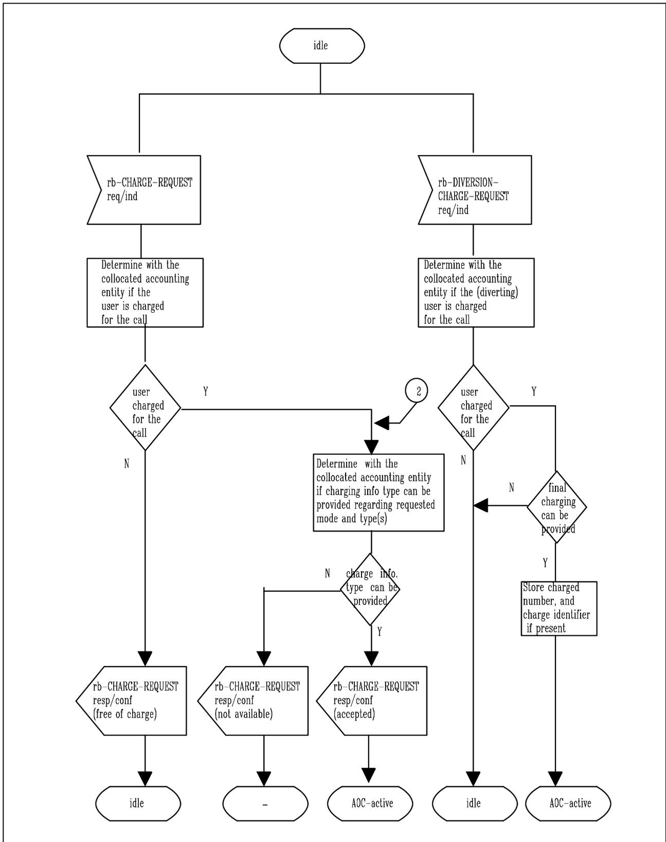
Figure 23 (part 1) - SS-AOC, SDL for functional entity FE3
