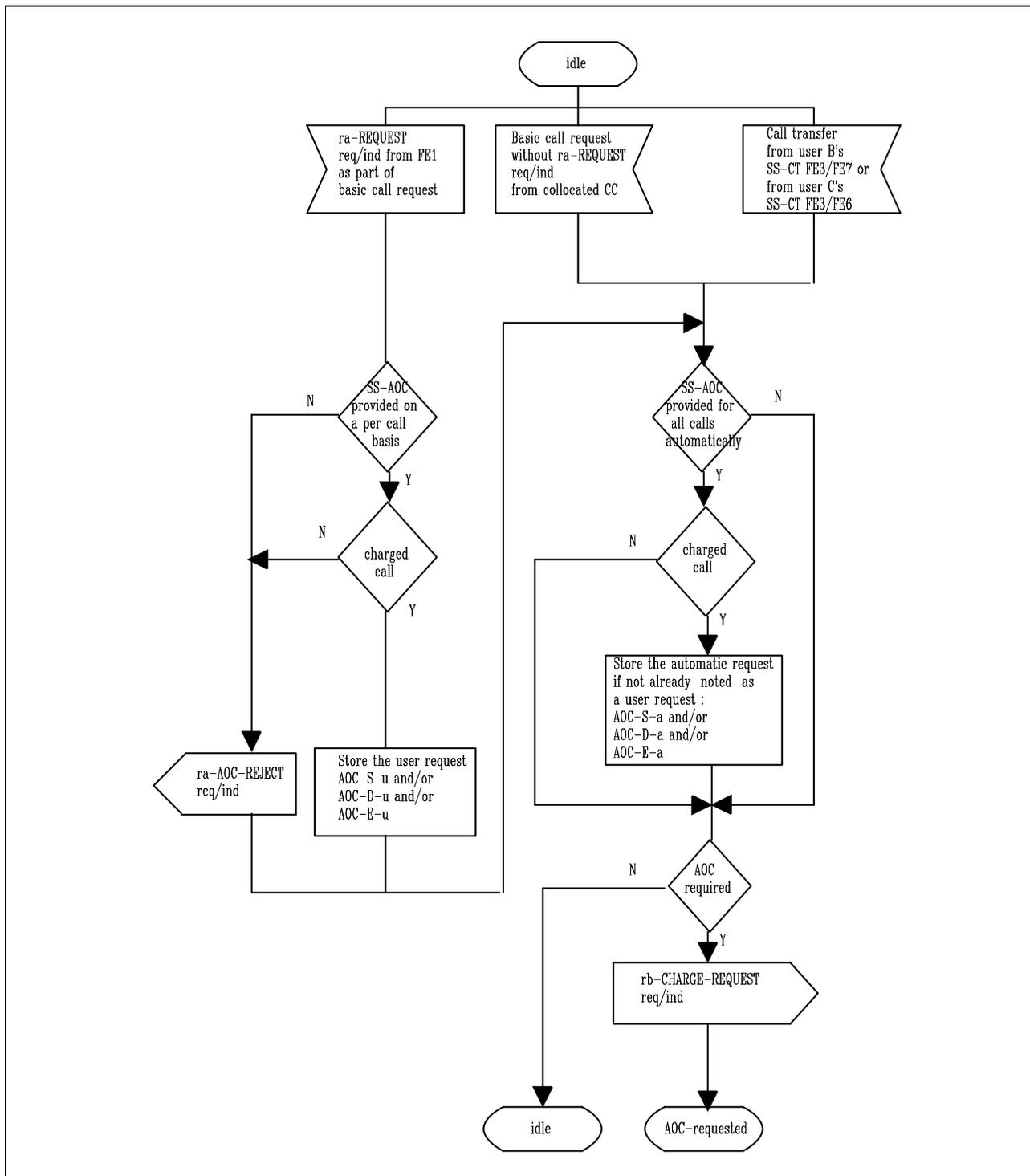
Figure 22 (part 1) - SS-AOC, SDL for functional entity FE2
