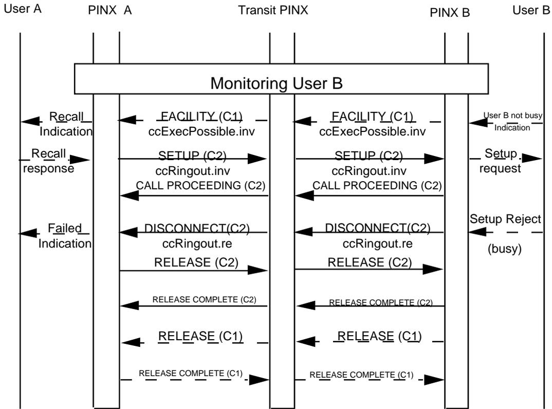
**Figure C.7 - Example Message Flow for User B Busy Without Service Retention**
