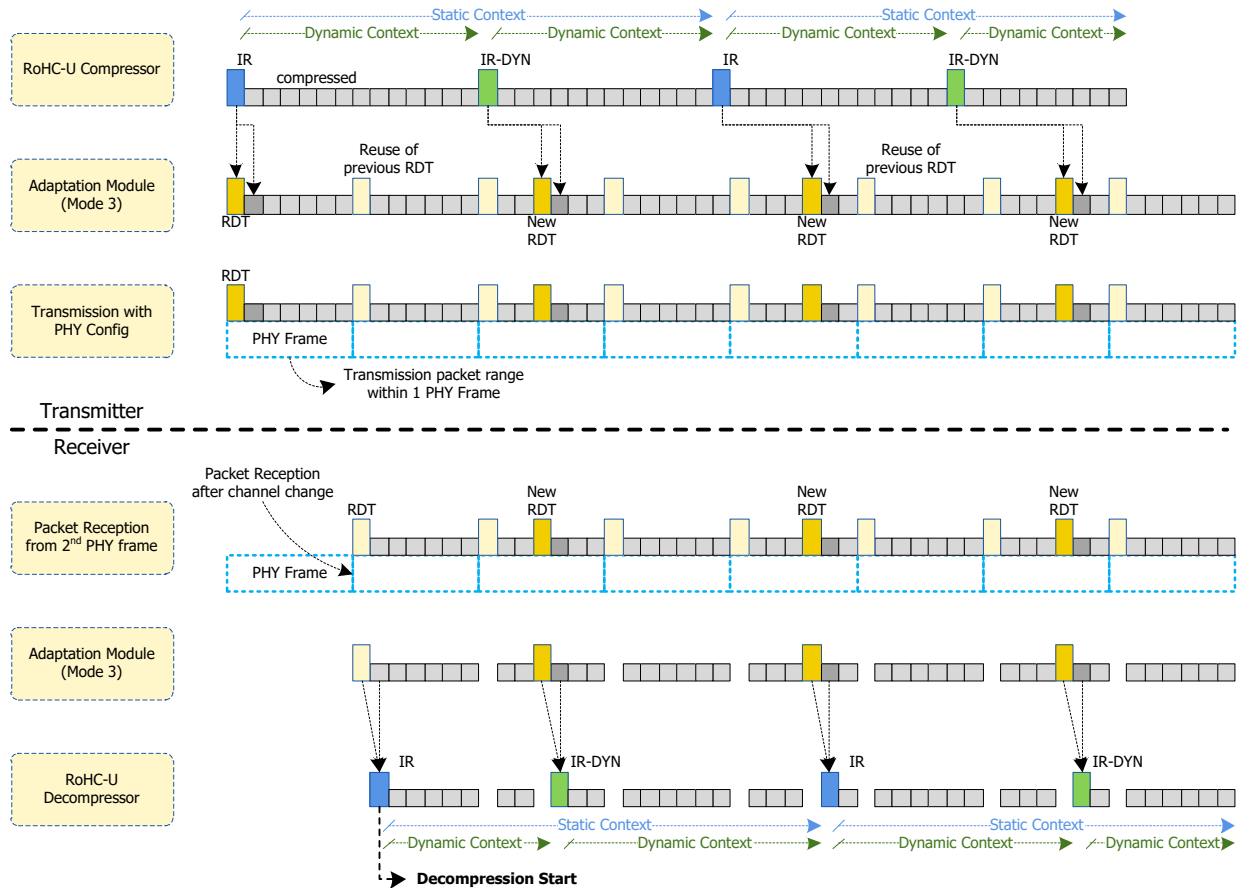
Figure D.3.1 Example of IP header compression using adaptation mode 3.
